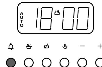
When the oven has switched off, **return the oven knob to the off position**, and press the *manual* button **(11)**.
