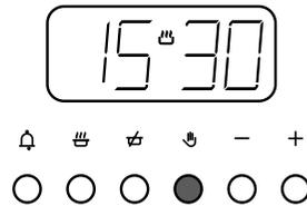
To set the programmer to manual operation at any time (cancelling any automatic setting), press the *manual* button. The programmer **must** be set to manual before the appliance can be used manually.
