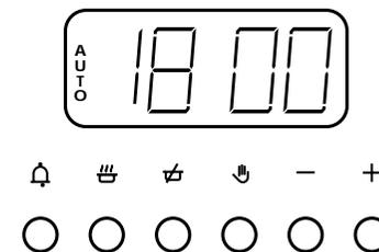
To switch off the alarm press the *minute minder* button **(10)**.
