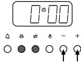
Press the *cook time* and *ready time* buttons simultaneously, and keep them depressed. Use the *plus* and *minus* buttons to set the required time.
