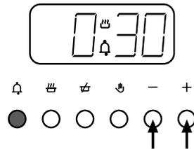
Press the *minute minder* button, then use the *plus* and *minus* buttons to set the required time.
