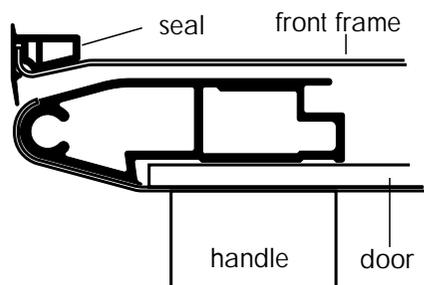
When securing the appliance, the fixing screws provided are driven through the edging strips into the cabinet - the seal will straighten up and sit flush to the cabinet when the screws are fully home.
