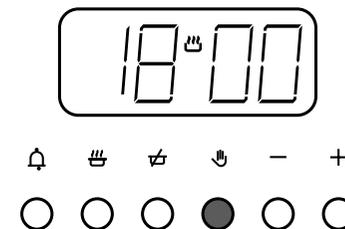
If you wish to cancel the automatic setting before cooking has started, and return to manual operation, press the *manual* button **(11)**. To cancel any remaining cooking time left on the clock before the alarm sounds, press the *manual* button **(11)**.
